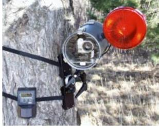
The TM700v Passive Infrared Video Trail Monitor can be easily mounted to a tree or post. This photo shows the TM700v mounted with the TM Video Camera, the TM Weather-Proof Video Enclosure, and the TM Video Light. The light is pictured here with the red light cover. Clear and infrared light covers are also available with the system.
